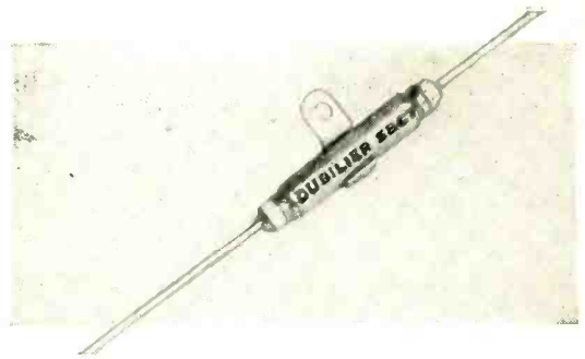
Fig. 4. Lead-through capacitor ( 0.005\mu\text{F} ) for suppressing interference on Band I from electric drills, etc.
